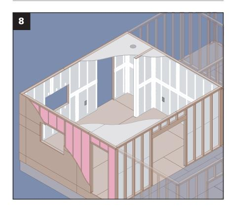
Apply joint compound to all corners, fasteners, and intersections, feathering it out to meet the paper face of the drywall. The third coat is slightly wider than the second coat. After sufficient drying, sand all areas covered with joint compound to ensure a smooth finish.
