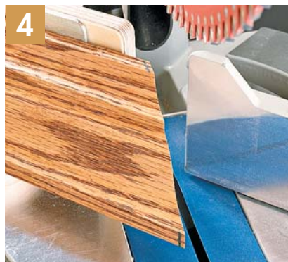
4 ▲ Adjust the saw angle to make a cut parallel to the two marks. Cut to the waste side. Readjust saw if needed.
