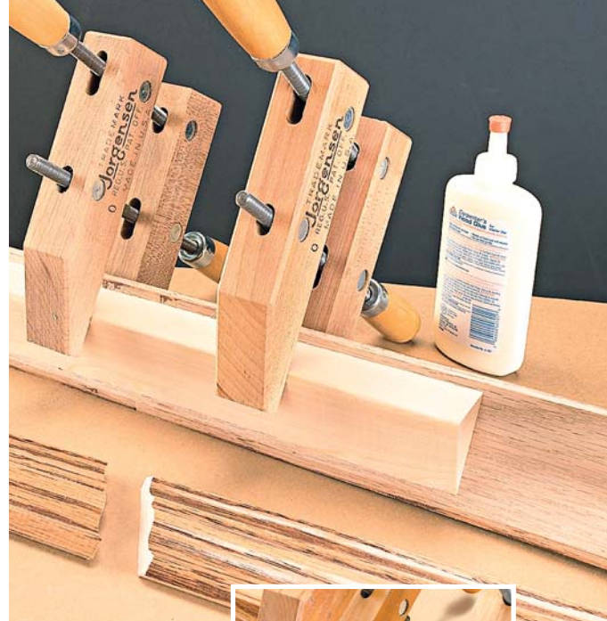
▲ A short length of backer adds rigidity when gluing a splice joint together. Careful attention to the grain makes for a virtually seamless joint ( right ).
