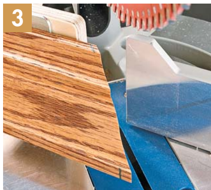
3 ▲ With the miter saw rotated to 45° (right or left) make a cut about 1/4" to the waste side of the layout lines.
