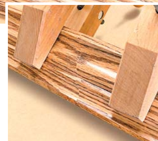
▲ A short length of backer adds rigidity when gluing a splice joint together. Careful attention to the grain makes for a virtually seamless joint ( right ).
